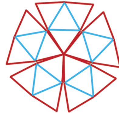
figure 1. Geodesic pattern – 2V Frequency Alternate Division based on Icosahedron symmetry [11].
