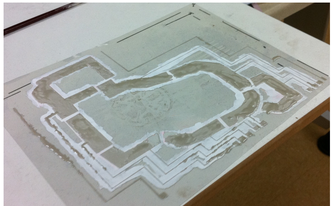
Figure 4: Printed dielectric (white) and conductive ink (silver)
