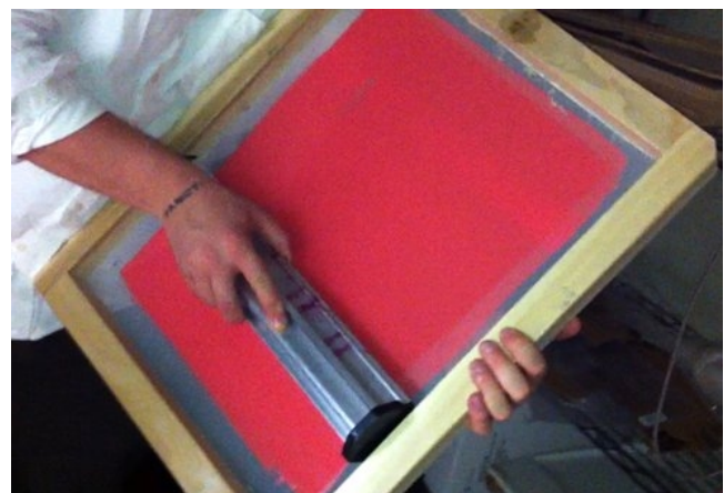
Figure 1: Applying photo emulsion to silk screen
